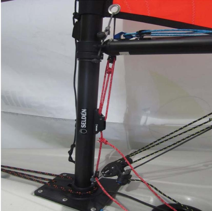
Also features a rope bobble (allowed) as a means of quick rigging (operates like the clew tie down)
