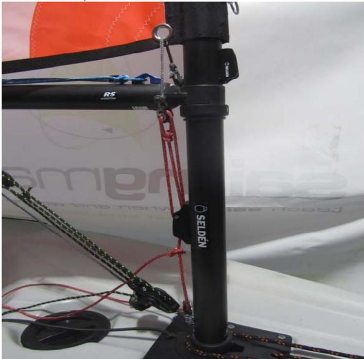
This downhaul system requires 1 extra block (so 2 in total), 2.5m of 4mm line, and a further 60cm of 4mm line at the top. If the easy rig option is required it is 40cm of 3mm line and a rope bobble or big knot in the end. (a rope bobble is considered a knot in a rules interpretation). This is knotted through the gooseneck moulding and round the mast for strength.
